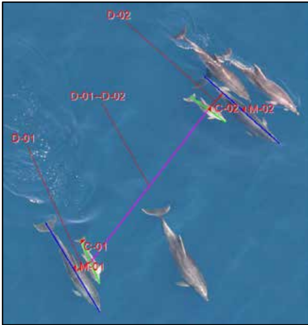
Fig. 3. Sample image showing an example of how Image-Pro v. 11 may be customized for UAV image analysis. After using the “Mother Line” (blue, M-01 & M-02) and “Calf Line” (green, C-01 & C-02) tools to measure and calculate calf size relative to its mother, distances between individuals can be calculated using “Distance between Centers” (red, mother-calf distance D-01 & D-02) and “Set to Set Distance” (magenta, calf-calf distance D-01-D-02) tools. Figure courtesy Matthew Batchelor, Alces Imaging and Automation, LLC. Image from https://www.onegreenplanet.org/wp-content/uploads/2014/08/bottlenosedolphin5_fullsize1.jpg
