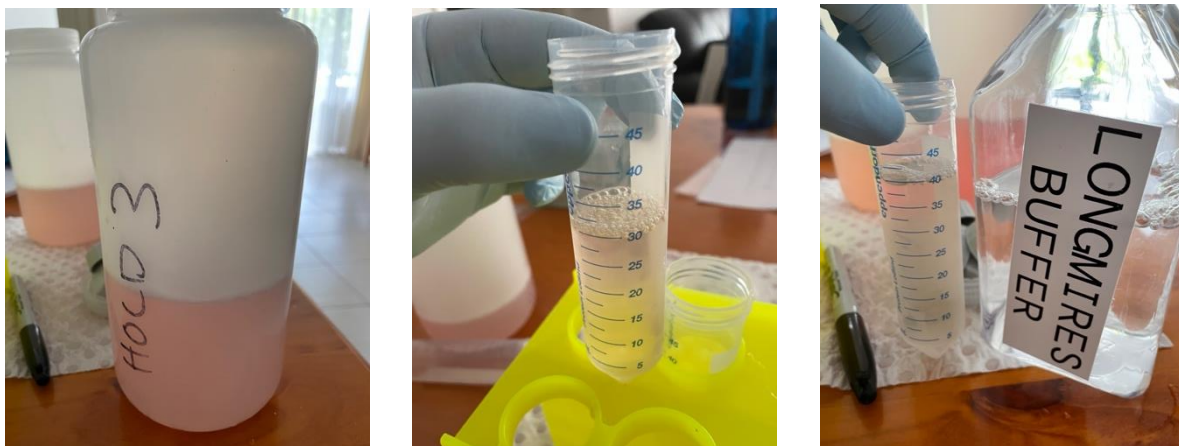
Figure 1. Process of decanting hold samples into preservation medium. Left- Sample collected from hold onboard fishing vessel. Middle- 30ml of sample poured into collection tube. Right- 10ml of Longmire Buffer added to tube for DNA preservation.
