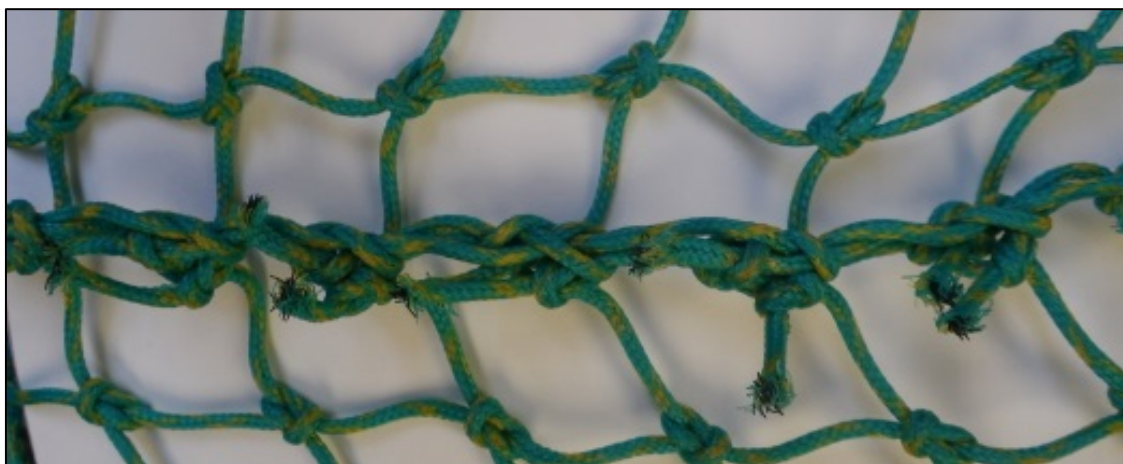
Figure 3. How the bar cuts are sewn together between the tails of the tube
