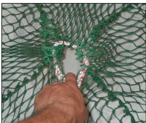
Figure 10. The spliced 3/8" nylon closer ring at the tail of the net
