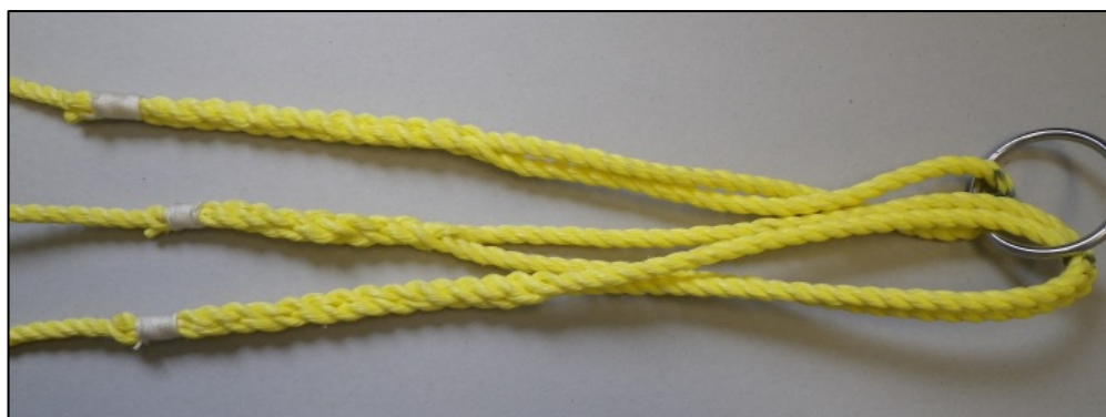
Figure 12. The lifting point at the top of the bridle
