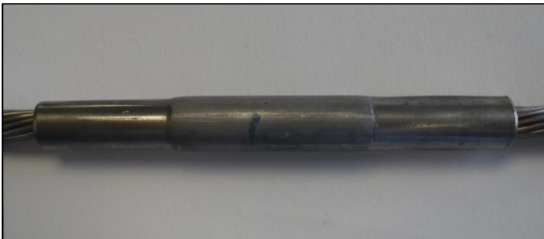
Figure 6. 4" pipe used to crimp the cable into a loop
