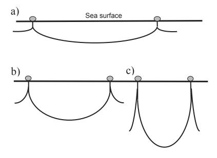
Figure 1. Stylised version of mainline configurations at fishing depth. Shown are a) surface set tight, b) surface set loose, and c) deep set loose mainlines.
