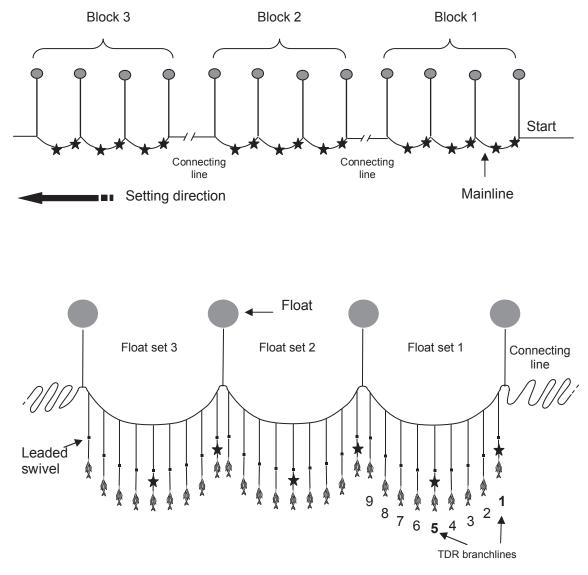
Figure 2. Gear configuration and position of time-depth recorder (TDR) branch lines used in the experiment. As indicated, each treatment of mainline tension comprised three float sets and each float set comprised two TDR positions.
