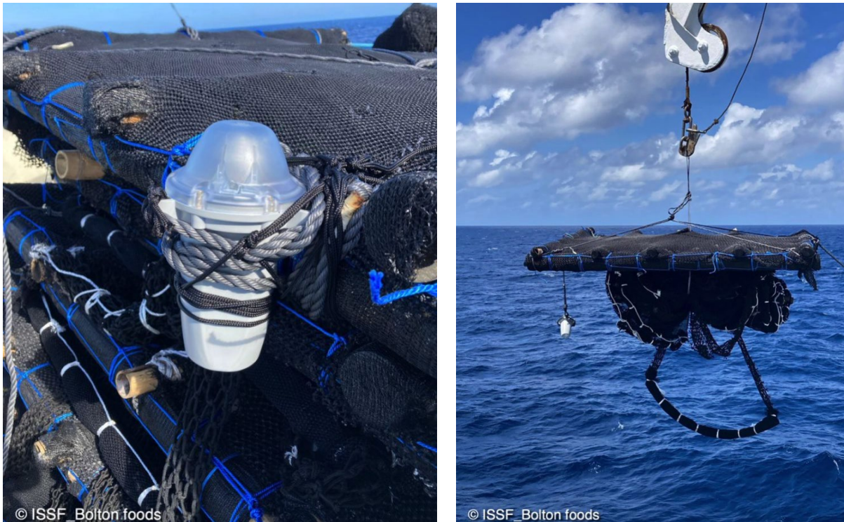
Figure 4 – Fixation systems: (left) directly to the FAD and (right) attached to the FAD with a rope.
