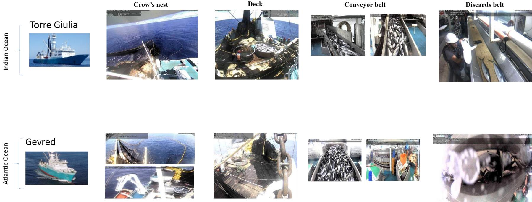
**Figure 1.** Details of EMS installation on *Torre Giulia* and *Gevred* CFTO vessels and global view from each camera.
