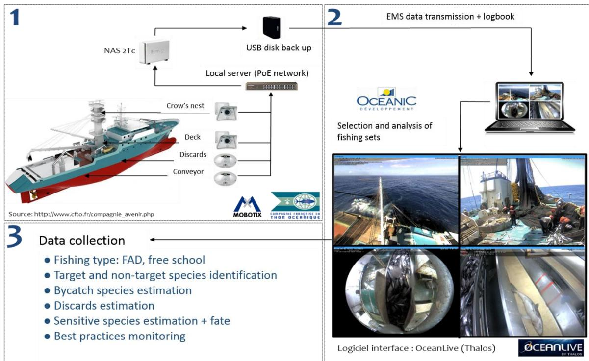
**Figure 2.** Schematic representation of the EMS installation and the process of data collection
