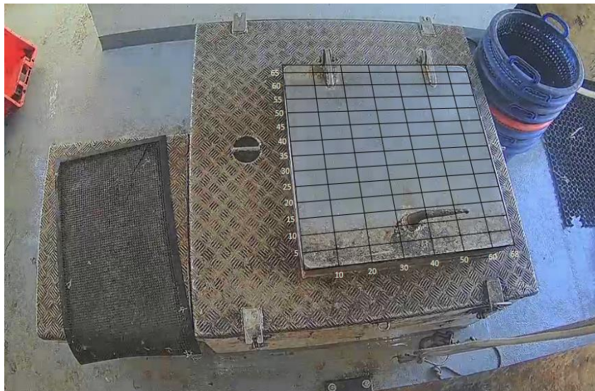
Figure 2: Example of a calibrated hatch onboard a commercial fishing vessel. These areas will vary from vessel to vessel, depending on available surfaces and the species being measured. This image is provided as an example from a non-tuna fishery. For tuna and tuna-like fisheries, the defined areas will have to be larger to accommodate larger species (image source: CEFAS).
