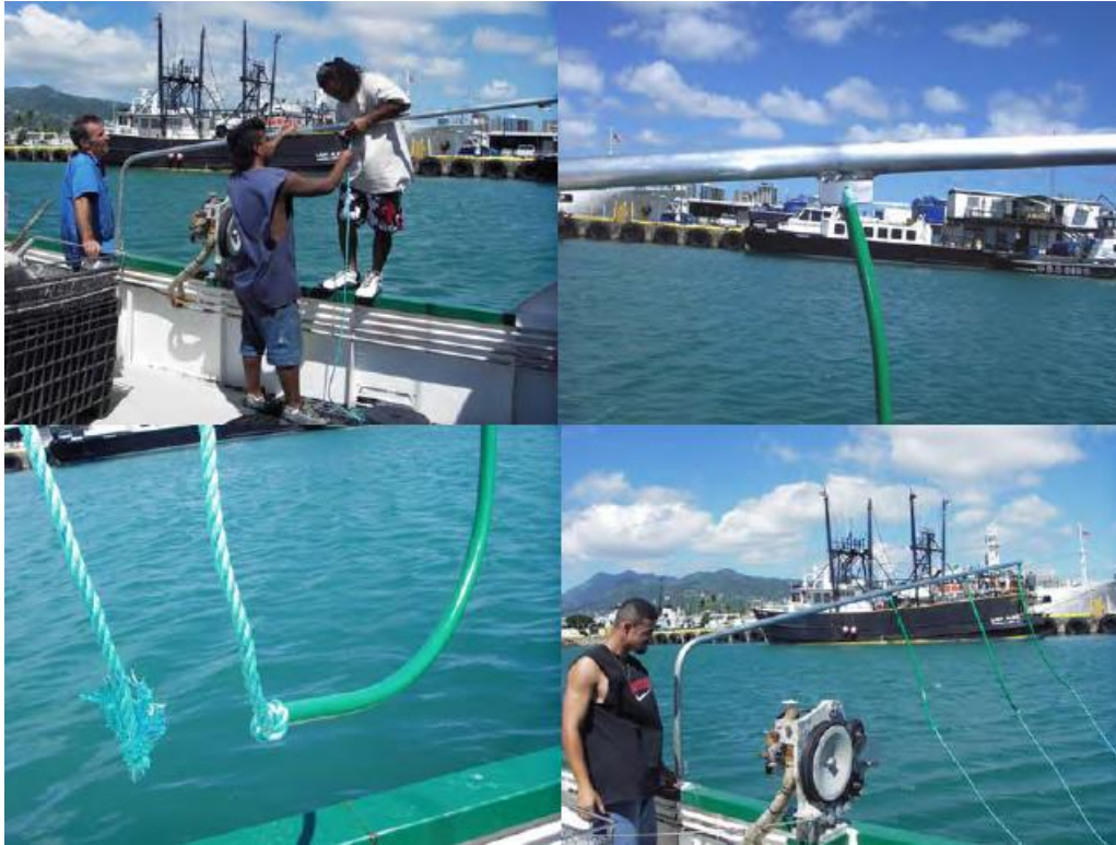
Fig. 1b. Installing a bird curtain for use during setting. Top left: attaching the streamers to the pole by either eye splicing through the 13 mm hole in the aluminum tab on the pole, or onto a stainless steel clip. Top right, attaching the streamer to the pole. Bottom left: knot holding the hose in place, either backsplicing or heat sealing the end of the streamer. Bottom right: a deployed bird curtain for use during side setting (Brothers and Gilman, 2006).
