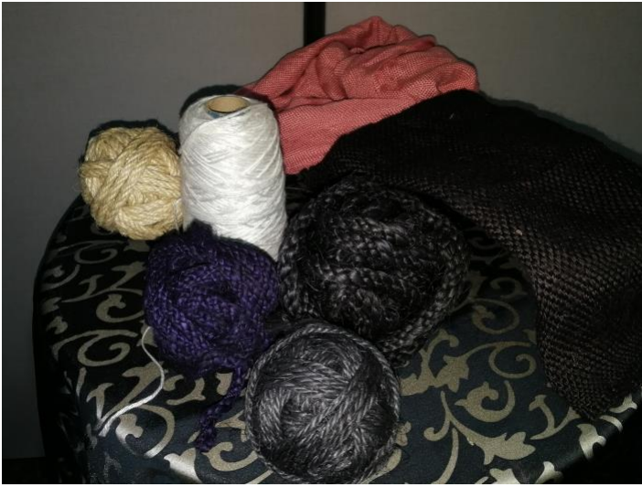
Figure 6. Biodegradable FAD materials: a) Bamboo twine (white), bamboo canvas (pink), and agave fiber rope (natural color and died black and dark blue); b) bamboo and balsa wood raft after 10 months in a seawater pool.
