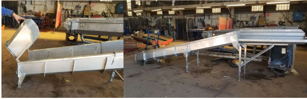
Figure 27 - Ramp with lifting end section for easy crossing (left) and an elevatable "table" section and adjustable legs to select the best height for bycatch release (right).
