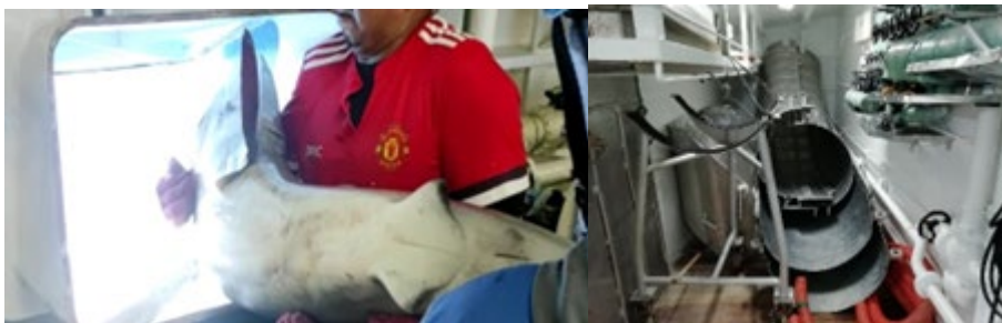
Figure 11 - Fishers manually moving sharks from the conveyor belt in the lower deck to the gutter (left) and mobile system with chute sections and wheeled supporting frames (right).
