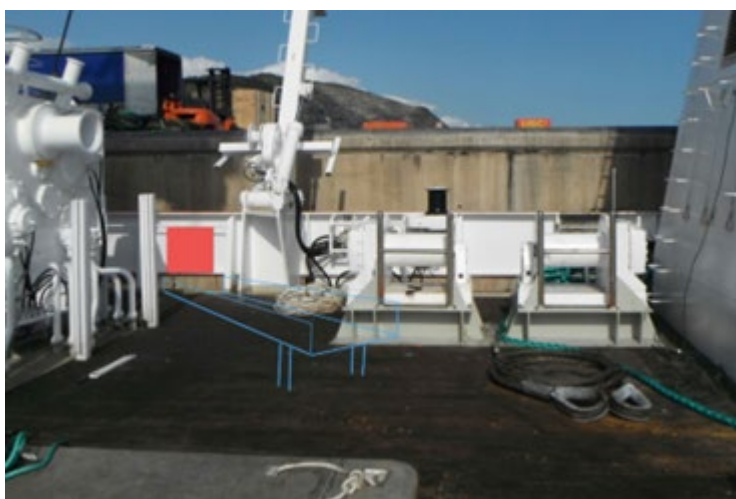
Figure 34 - Proposed door opening (red square) to install a straight release ramp, as the two chokers obstruct the passage to the door already in place.
