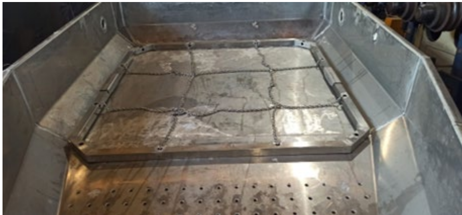
Figure 6 – Mobulid sorting grid fitting inside the tray of a hopper.
