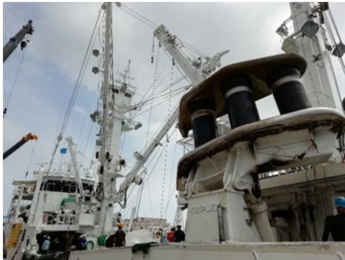
Figure 32 - Triplex net hauling system in a modern tuna purse seiner at the port of Yaizu (Japan).
