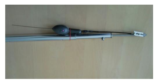
**Figure 1.** Configuration of tag ready for deployment in the Escalle et al. (2014) study showing 4-meter tagging pole, applicator pin, titanium anchor, 20 cm tag tether, and miniPAT tag with rubber band.
