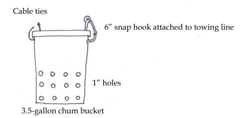
Figure 7. Chum bucket. About 2 gallons (10 lbs) of chum are place in the bucket and the lid is secured shut with towing hook and cable ties.
