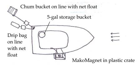
Figure 9. Speedboat with bait station components: 3.5-gallon chum bucket, drip bag for fish oil, Mako Magnet sound attractant. Chum bucket and drip bag are placed in 5-gallon storage bucket when not deployed.
