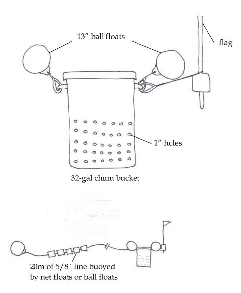
Figure 11. Drifting chum bucket (Alternative 5). The buoyed line allows the bucket to be lowered over the side of the seiner and retrieved. A longer line would allow the bait station to be tethered to the seiner if desired.
