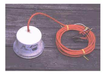
Figure 8. Transducer and power cable of Mako Magnet sound attractant. The transducer will be placed inside a plastic storage crate, cable-tied to the bottom of the crate, with the cable side up. The storage crate will be secured to the side of the boat; the cable will be connected to either the boat's battery or an auxiliary battery.
