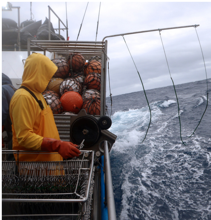
Bird curtain that has been deployed to prevent seabirds from landing on the water where bait is accessible.
