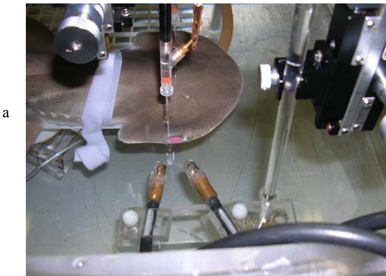
Figure 8.—The electroretinogram apparatus used to measure the response of sharks to various wavelengths of light.
