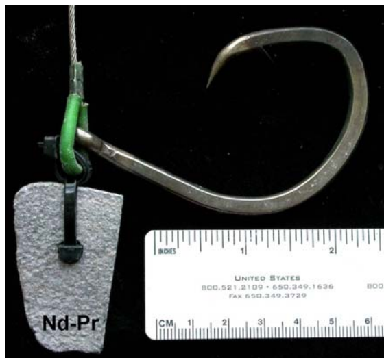
Figure 2.—Example of how a rare earth metal alloy is deployed on a long line circle hook to present an electric field in seawater sufficient to deter sharks from biting at the bait on the hook. The Nd-Pr alloy generates a measurable electric field in seawater. However, the close proximity of the Nd-Pr alloy to a stainless steel cable leader and a galvanized steel circle hook presents the challenge of numerous potential galvanic interactions.
