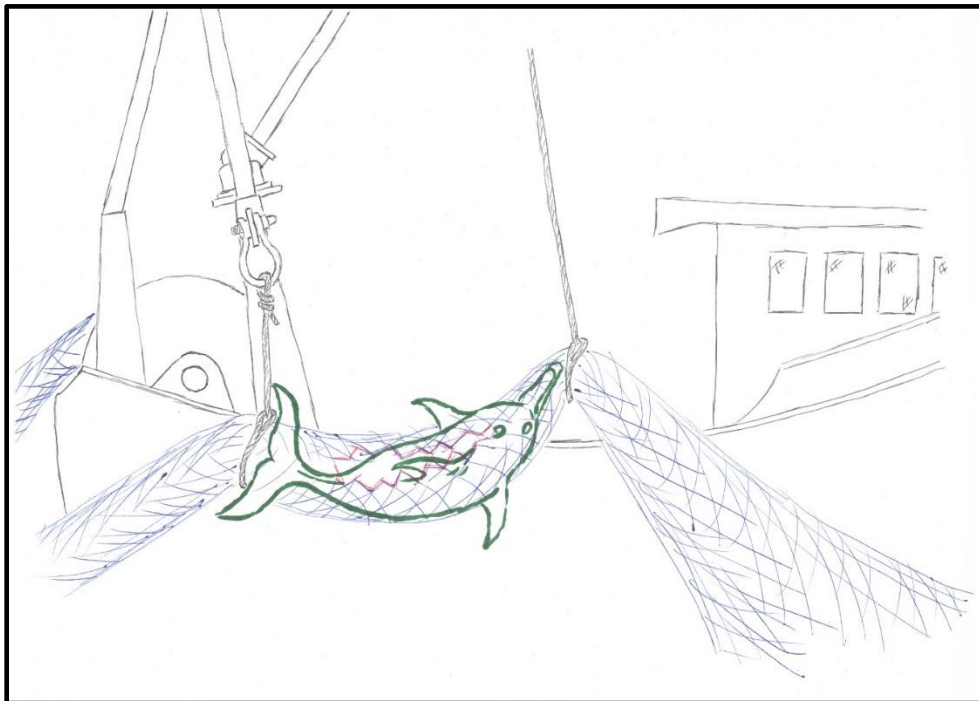
Figure 7a. Releasing small cetacean trapped in the 'sweep' of a trawl net of a small trawler. When a small cetacean is bycaught in the large meshes at the front of the net, hauling should slow so that the animal can be brought alongside. A combination of ropes and the crane should be used to hold it in place, so the meshes can be carefully cut to facilitate its release.
