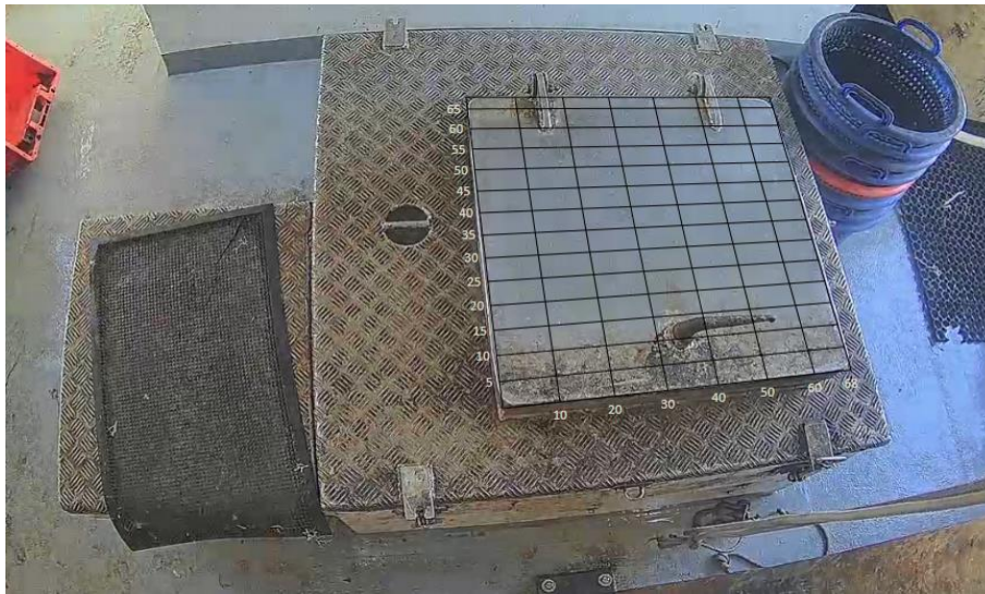
Figure 1. Example of a calibrated hatch onboard a commercial fishing vessel. These areas will vary from vessel to vessel, depending on available surfaces and the species being measured. This image is provided as an example from a non-tuna fishery. For tuna and tuna-like fisheries, the defined areas will have to be larger to accommodate larger species.
