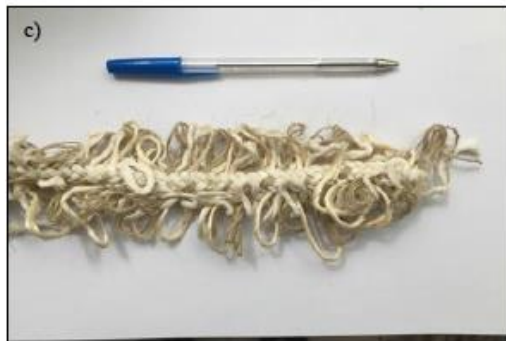
Figure 18.2. Selected ropes for the experiment: a) cotton rope; b) sisal and cotton rope; c) cotton, sisal and linen rope with loops.
