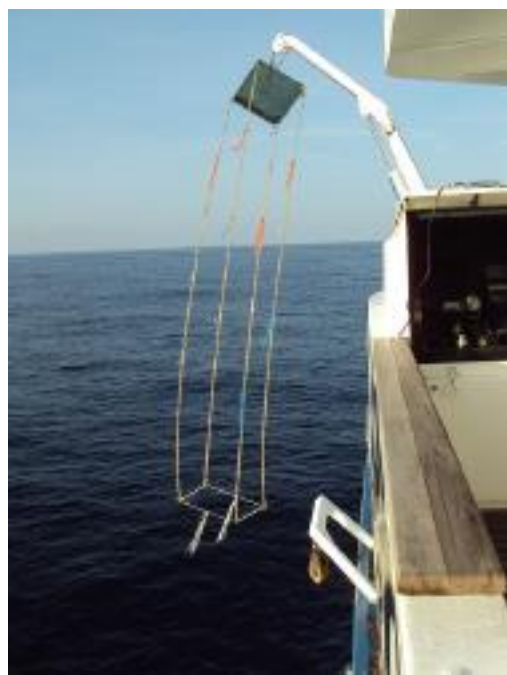
Figure 19.1. FAD design type 1: used at 10m and 30m depth
