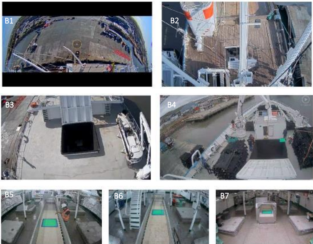
Figure 1. (A) An example of a 6-camera EM system installed in a purse seine covering main areas of fishing and fish handling operations (from Murua et al., 2020b) and (B) 7-camera EM system (4 in the upper deck and 3 in the well deck) installed in a purse seine covering main areas of fishing and fishing handling operations including 1 more camera in the conveyor belt: (B1) 360° Panoramic view camera (e.g port side view), (B2) Crows nest stern view camera, (B3) Working deck crane camera view , (B4) Foredeck view camera, (B5) Conveyor belt stern camera view, (B6) Conveyor belt middle camera, and (B7) Conveyor belt bow camera (source: Digital Observer Services).
