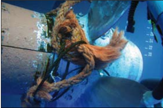
FIGURE 8 The effects of ALDFG on propellers
