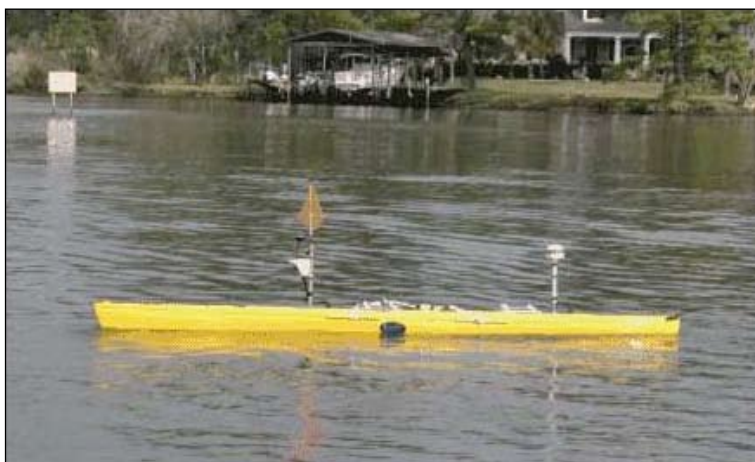
FIGURE 13 Autonomous survey vessel used in the Gulf of Mexico
