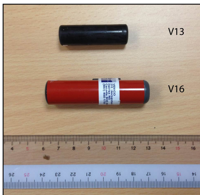
Figure 2.5 Acoustic tags used during the study of silky sharks associated with drifting FADs in the western Indian Ocean. The upper tag is a coded V13, while the lower (red) tag is a continuous V16P tag.
