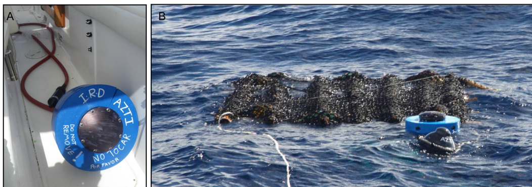
Figure 2.4 VR4-Global acoustic receiver (A) prior to deployment with hydrophone configuration and (B) deployed on a drifting FAD alongside a grey GPS echo-sounder buoy.
