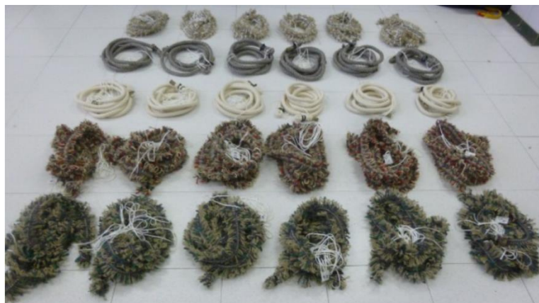
Figure 32. Pictures of the 5 different biodegradable twines tested by Lopez et al. (2016, 2019)
