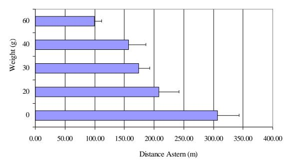
Figure 5. Estimated distance astern at which baited hooks sink to a benchmark depth of 10 m at a speed of 9.5 knots over ground. Error bars are 95% confidence intervals.
