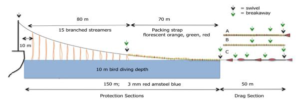
Figure 1. Schematics of tori lines. Light tori line (above) and hybrid tori line (bottom). Bird access zone is the distance astern baited hooks are above 10 m depth which was assumed to be 150 m for unweighted branchlines.
