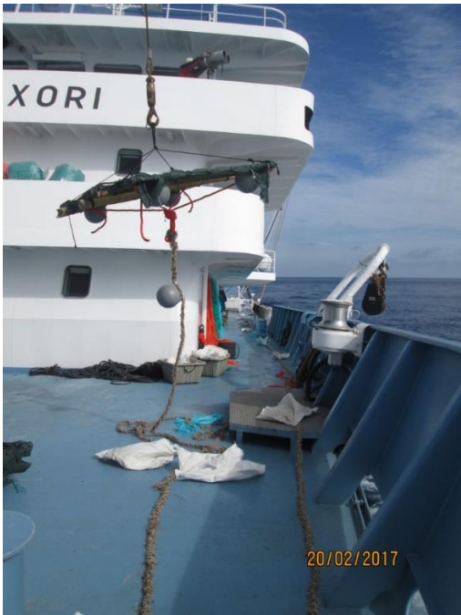
Figure 2. FAD type 1: 4 biodegradable cotton ropes hanging from the raft. This design was used at 10 m and 30 m depth.
