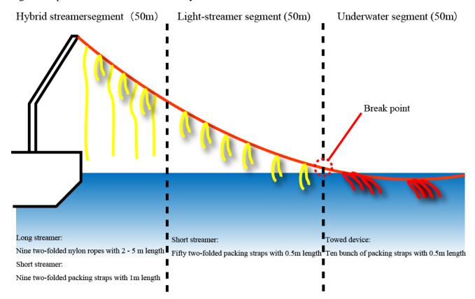
Figure 1 Specification of the modified hybrid tori line
