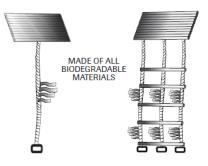
In addition to having minimal risk of entanglement, they are constructed exactly like other non-entangling FADS, but using only natural and/or biodegradable materials, further reducing the environmental impact of DFADs on the oceans
