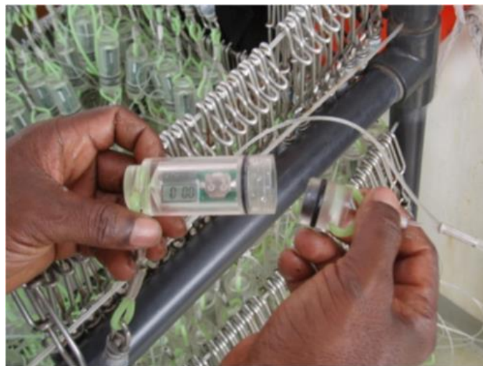
Figure 3. Photo showing hook timers (HT) developed by Somerton et al. (1988). The HT is attached at the top of each branchline and is triggered by the attack of the bait by a predator and therefore indicates the elapsed time between the hooking contact (with success or not) and the hauling of the hook (with capture or not) on the deck.
