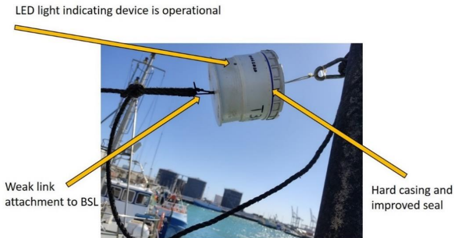
Figure 4. Image showing improvements made to the casing and device to withstand the harsher conditions on Trawl vessels.
