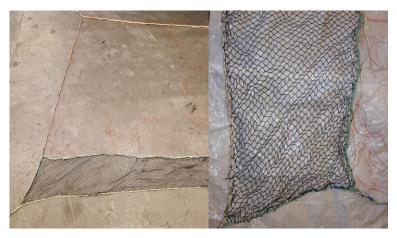
Figure 2. Pictures of the modified gillnet where a small dark meshed net is attached to the bottom part of a standard net. Left: zoomed out. Right: zoomed in on the lower part.
