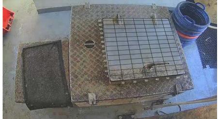
**Figure 1.** Example of a calibrated hatch onboard a commercial fishing vessel. These areas will vary from vessel to vessel, depending on available surfaces and the species being measured. This image is provided as an example from a non-tuna fishery. For tuna and tuna-like fisheries, the defined areas will have to be larger to accommodate larger species.
