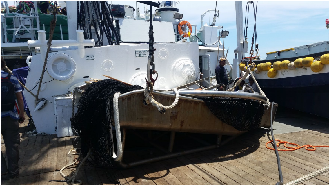
Figure 6. Hopper and brailer on the top deck of a purse seiner while at port in Majuro (Marshall Islands, 2018).
