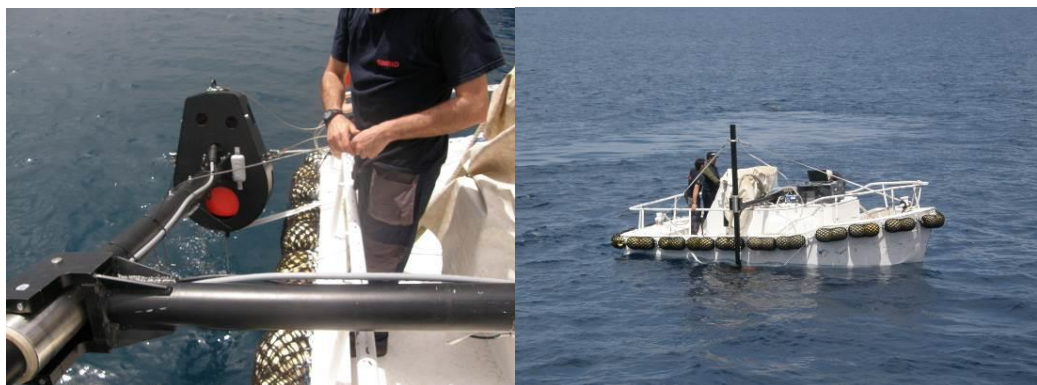
Figure 3. Scientific echo-sounders installed on the work boat ("panguita").
