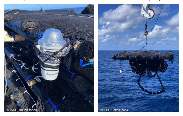
Figure 4 – Fixation systems: (left) directly to the FAD and (right) attached to the FAD with a rope.
