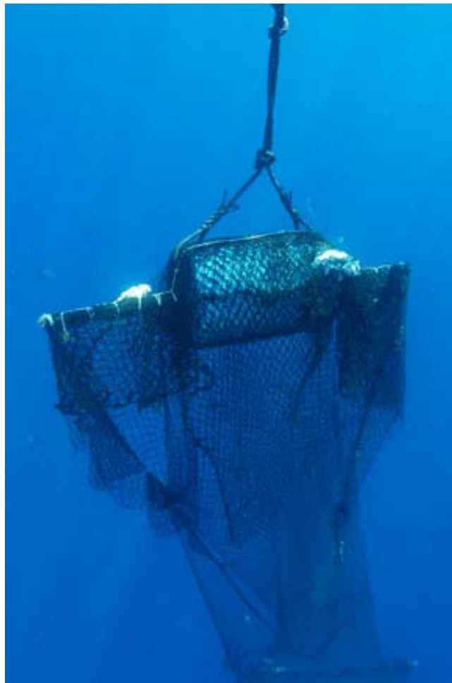
Fig. 9. Subsurface FAD built with a drum (© Fadio/IRD/Ifremer/mtaquet).
