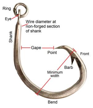
**Fig. 2** Hook minimum width and other main elements of a fishing hook (Curran and Bigelow 2011; Serafy et al. 2012). The part of the hook with the narrowest width varies by hook type as well as, to a smaller degree, for hooks of the same hook manufacturer and size
