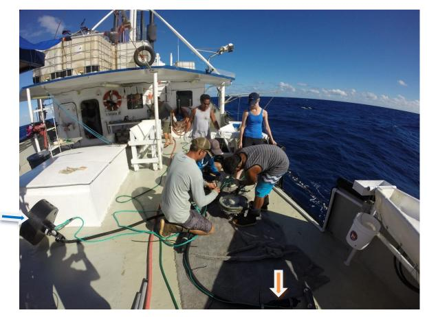
Picture 5: Attaching a VR4 receiver to a dFAD. Blue arrow shows the unit and orange arrow the hydrophone
