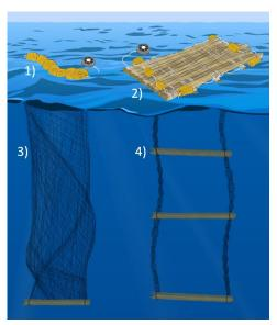
**Figure 2.** Diagram representing the most common dFAD designs in the WCPO. DFAD rafts are often made of: 1) several purse seine corks tightly wrapped in purse seine nets; or 2) a bamboo raft, with or without purse seine corks and covered by purse seine nets. The submerged appendages are typically: 3) open panels of purse seine nets; or 4) purse seine nets rolled up in a sausage and separated by bamboos.
