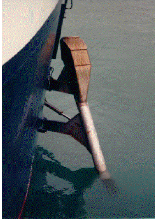
Figure 13. An underwater setting funnel, when not in use is turned and stowed against the hull
