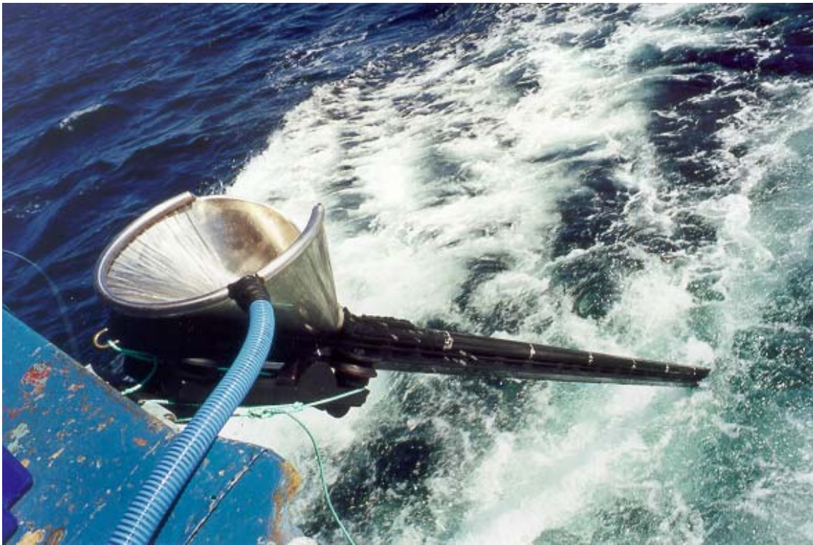
Figure 14. Underwater setting chute (New Zealand development system)
