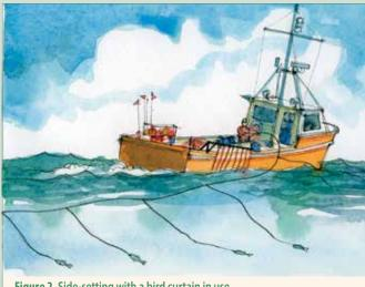
Figure 2. Side-setting with a bird curtain in use.
