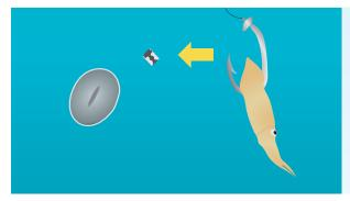
The shield increases the sink rate of the baited hook (without the need for lead swivels) and releases at a depth below the feeding range of seabirds and turtles.
