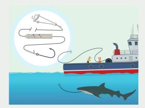
Fishermen can be injured by weights when the line suddenly breaks. Inset shows a sliding weight, a new weighting system developed to reduce the risk of injury.
