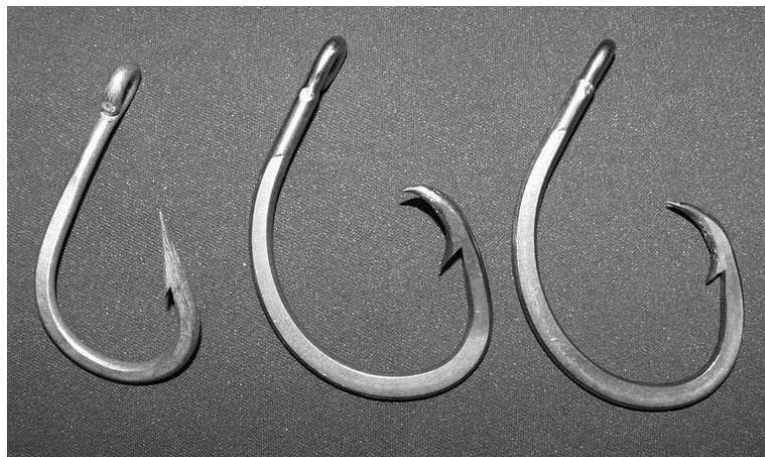
Figure 3. Comparison of hook designs; from left to right: 9/0 “J” hook with 25° offset, 18/0 circle hook with 10° offset, and 18/0 circle hook with 0° offset.
