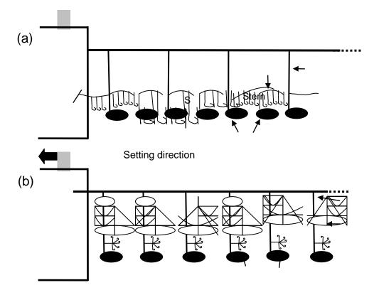
**Figure 1**. Typical configurations of the traditional Spanish double line system (a) and Chilean (trotline) system (b) showing differences in gear design and location of weights in relation to hooks. The open-ended secondary/connecting lines (not joined by a continuous hook line) and proximity of weights to hooks of the Chilean system enables hooks to sink rapidly and with a linear profile (no lofting in propeller turbulence) from the surface close to vessel sterns. Drawings not to scale.
