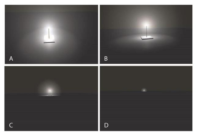
Figure 21 Modelled changes in the visibility of an unshielded 1000 W white LED viewed from A. 10 m; B. 100 m; C. 1 km and D. 3 km.
