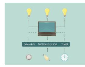
Figure 10 Use adaptive controls to manage light timing, intensity and colour.
