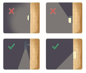
Figure 13 Lighting should be directed to ensure only the intended area is lit. Figure adapted from Witherington and Martin (2003)<sup>3</sup>.
