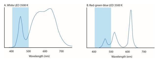
Figure 24 A comparison of the blue wavelength spectral content of two LED lights with the same CCT (3500k). The blue band shows the blue region of the visible spectrum (400–500 nm). The light in A has a much greater blue light content than B yet the two appear to the human eye as the same colour. For animals with differing sensitivities to light wavelength from humans, they may appear very different. Figure courtesy of lan Ashdown.
