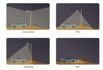
Figure 14 Lighting options for a parking area. Figure adapted from Witherington and Martin (2003)<sup>3</sup>.
