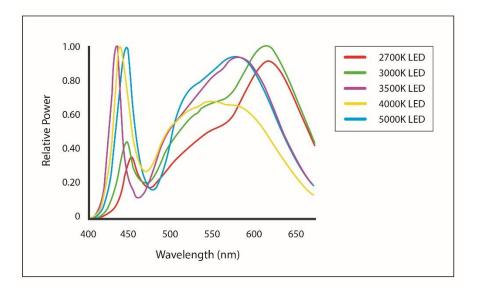
Figure 23 Spectral curves showing the blue content of white 2700-5000 K LED lights. Note the difference in relative power output in the blue (400 - 500 nm) wavelength range. Figure courtesy of lan Ashdown.
