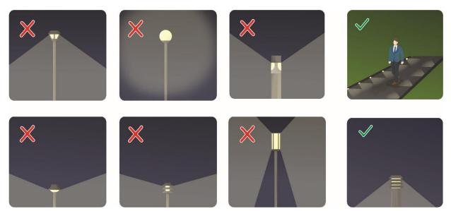
Figure 12 Walkway lighting should be mounted as low as possible and shielded. Figure adapted from Witherington and Martin (2003)<sup>3</sup>.
