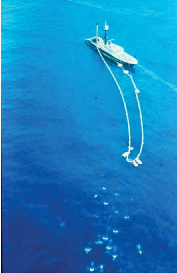
Fig. 2. The backdown manoeuvre used to release dolphins from tuna purse seines in the Eastern Pacific.
