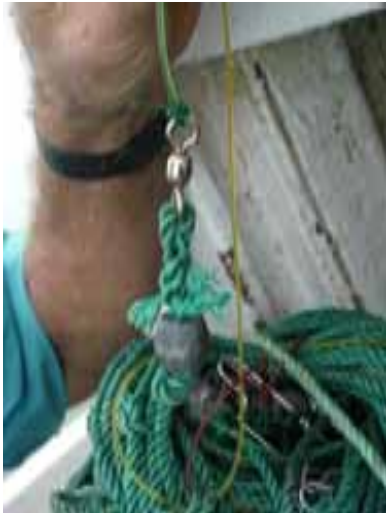
Here you see the branchline material, monofilament leader and separate weights and swivels.
