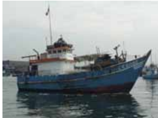
Longline vessel in Chimbote that had installed a mainline spool forward of the cabin in the dark area visible in the photo.
