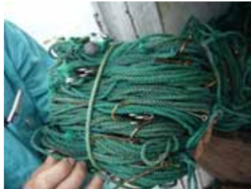
A branchline bundle from the Chimbote vessel.
