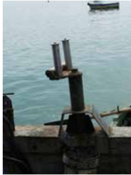
An example of a mainline puller and guide from a longline vessel in the port of Ancon.
