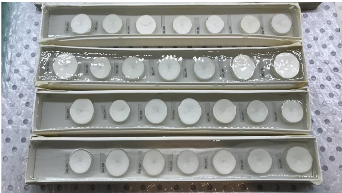
Appendix Figure 2. Larger BSH vertebrae in FAS channel moulds being embedded in casting resin.
