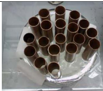
Paper tubes are sealed at one end with rapidly-cooled polymer
