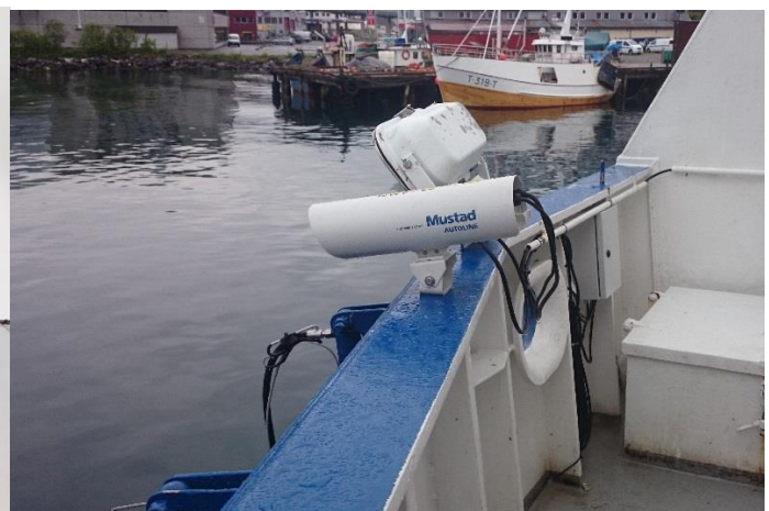
Seabird Saver laser system mounted on a Norwegian longliner.
