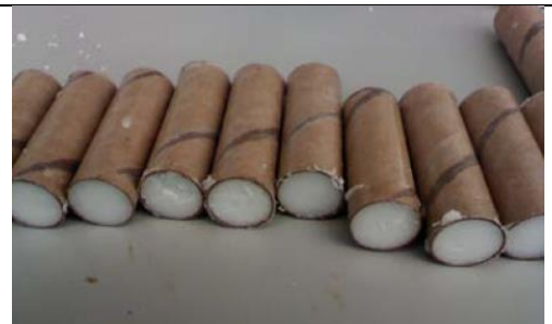
Once cooled, Polyshark is a hard solid in air, and stores indefinitely.
