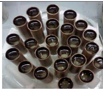
Molten polymer with repellent is poured into the tubes and cooled quickly
