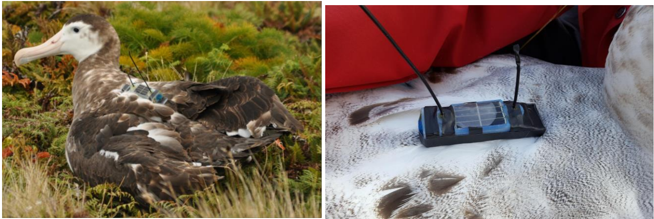
Figure 11. Above left, an adult female Antipodean wandering albatross with an Xargos transmitter taped to her back feathers. This was the first transmitter taped on and all subsequent Xargos transmitters were modified (above right, on male albatross) by shortening and re-sealing the plastic ends of the transmitters and reconfiguring the taping for more feather/tape/transmitter contact whilst still leaving the solar panel exposed to the sun.
