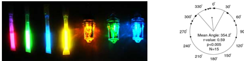
Figure 1.--Lightsticks tested in behavioral experiments. Essentially all colors and types of activated light attracted turtles to orient towards the light source (0°).
