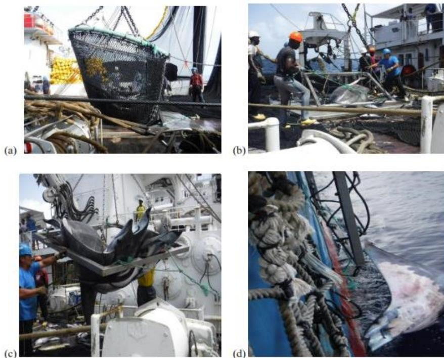
**Figure 11.** Mobulid sorting grid operation sequence showing the release of three adult Chilean devil rays (*Mobula tarapacana*) simultaneously over the starboard (Albacora/AZTI ©).
