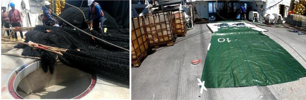
**Figure 10.** Small deck with little space for a hopper during net hauling (left) and hopper tarpaulin template to discuss with skipper preferred design and location on deck (Pevasa/Calvo/AZTI ©)
