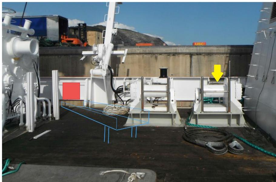
**Figure 7.** Starboard upper deck door (yellow arrow) behind two chockers and suggested new “cat flap” opening (red square) on sidewall to facilitate releases with a straight ramp.
