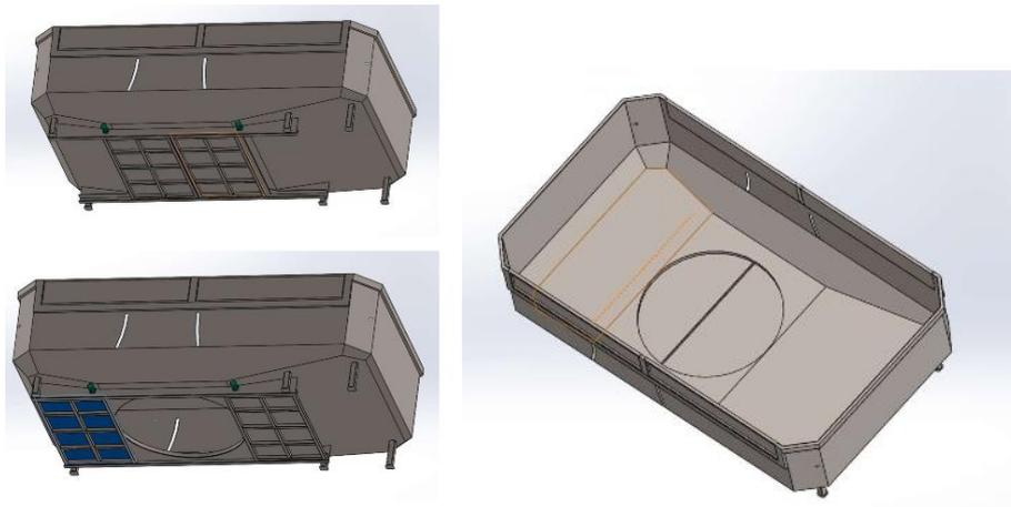
**Figure 9.** Lower and top view of integrated hopper desing with opening door to control bycatch releases from the upper deck
