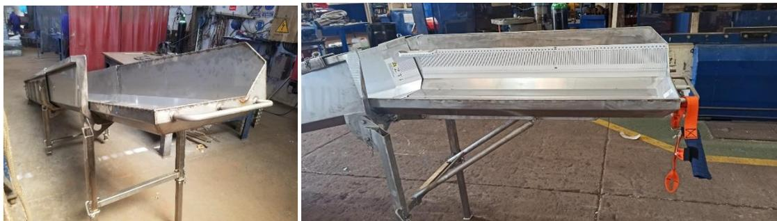
**Figure 6.** Retractable ramp and adjustable height with horizontal initial section to deposit and measure bycatches (Jealsa/AZTI ©).
