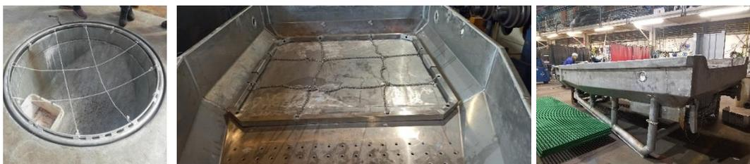
**Figure 12.** Round sorting grid on unloading hatch (left) and square sorting grid extended on hopper tray (middle) and stored folded underneath (right) (Pevasa/Jealsa/AZTI ©).
