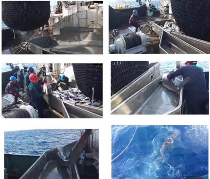
**Figure 8.** Shark release sequence using mobile hopper with ramp positioned on the starboard (Bolton Group/AZTI ©).
