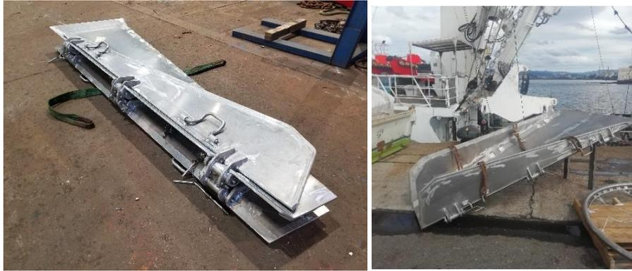
**Figure 5.** Release ramp folded for easy storage and extended for working (Pevasa/AZTI ©).
